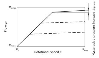
Characteristic curve valid at  $n_1$  = 1500 rpm and  $\theta_{fluid}$  = 50 °C.
