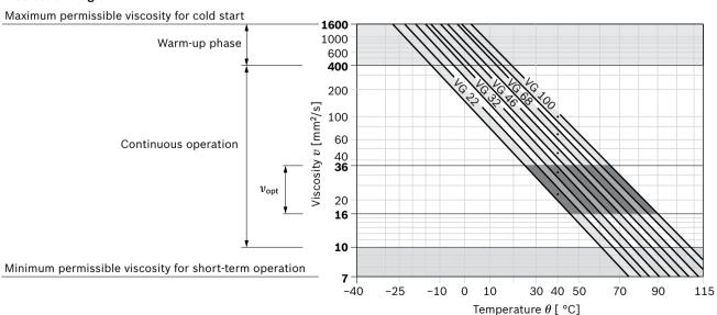
$_{\mbox{\scriptsize 1)}}$  Corresponds e.g. for VG 46 to a temperature range of +4 °C to +85 °C (see selection diagram)
