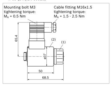
The seal ring in the cable fitting is suitable for lines of diameter 4.5 mm to 10 mm.
