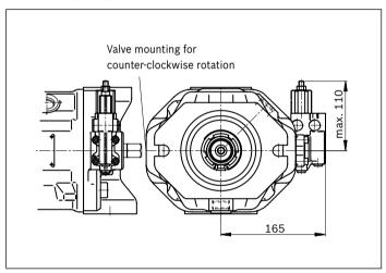
**▼** DRG - Pressure controller, remote controlled
