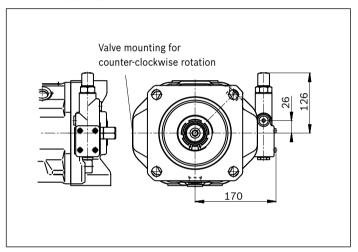
**▼** DRG - Pressure controller, remote controlled
