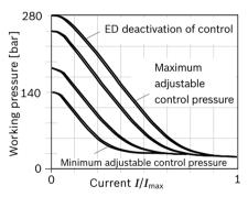
► Hysteresis static current-pressure characteristic curve < 3 bar.
