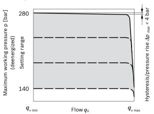
Characteristic curves valid at  $n_1$  = 1500 rpm and  $t_{fluid}$  = 50 °C. Control fluid consumption: 3 to 4.5 l/min.
