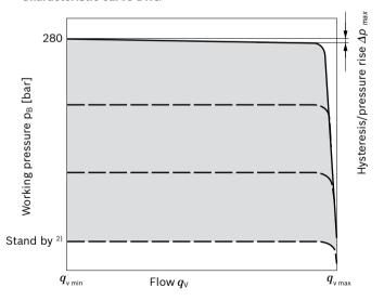
Characteristic curve valid for  $n_1$  = 1500 rpm and  $t_{fluid}$  = 50 °C.
