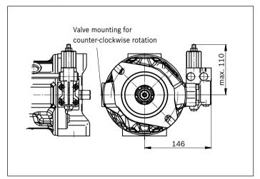
▼ DRG - Pressure controller, remote controlled
