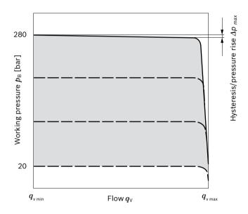
Characteristic curve valid at  $n_1$  = 1500 rpm and  $\theta_{fluid}$  = 50 °C.
