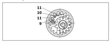
The radial compensation elements consist of segment (9), segment support (10) and seal rolls (11).
