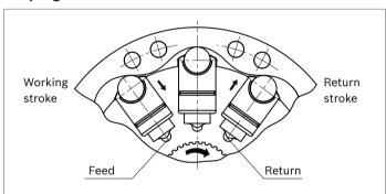
The number of working and return strokes corresponds to the number of lobes on the cam multiplied by number of pistons in the cylinder block.
